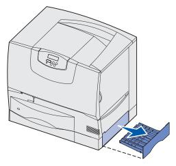
2 Remove any jams and then reinstall the tray.
